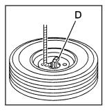
Put the tire on the ground at the rear of the vehicle with the valve stem pointed down and toward the rear of the vehicle.
